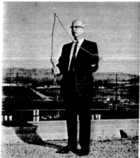
Figure 1. The early dowsing experiments utilized a single strain gauge bending beam holding one leg of the forked twig, with the human carrier (author) supporting the other leg in the palm of his hand.
